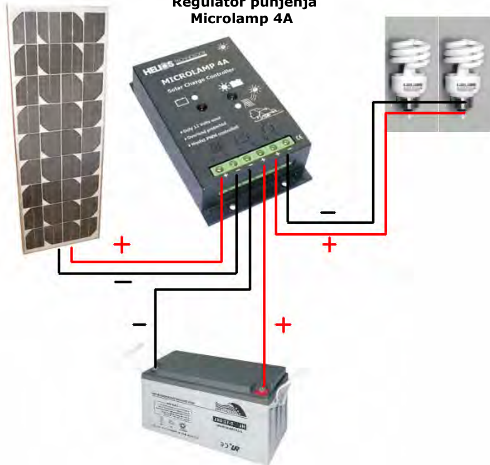
Solarni akumulator HL46Ah, 12VDC, C100
